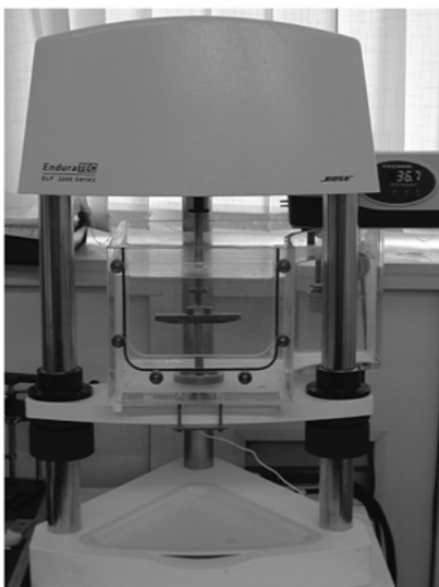
Figure 1 Mechanical setup system. The phase angle is independent of the specimen geometry and equals to the phase angle between the controlled or input signal (the displacement) and the monitored or output signal (the load).
